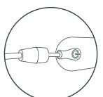
Insert the charging pin through the rubber into the port. The rubber will stretch open to accomodate the pin. It's a tight fit!
